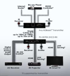
Input: 1x RJ45 (1x HDBaseT HDMI & Propriety Data)
